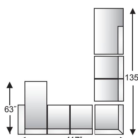
Dimensions are based on model L5002. For model L5003 add 1" per arm to the length dimension.
